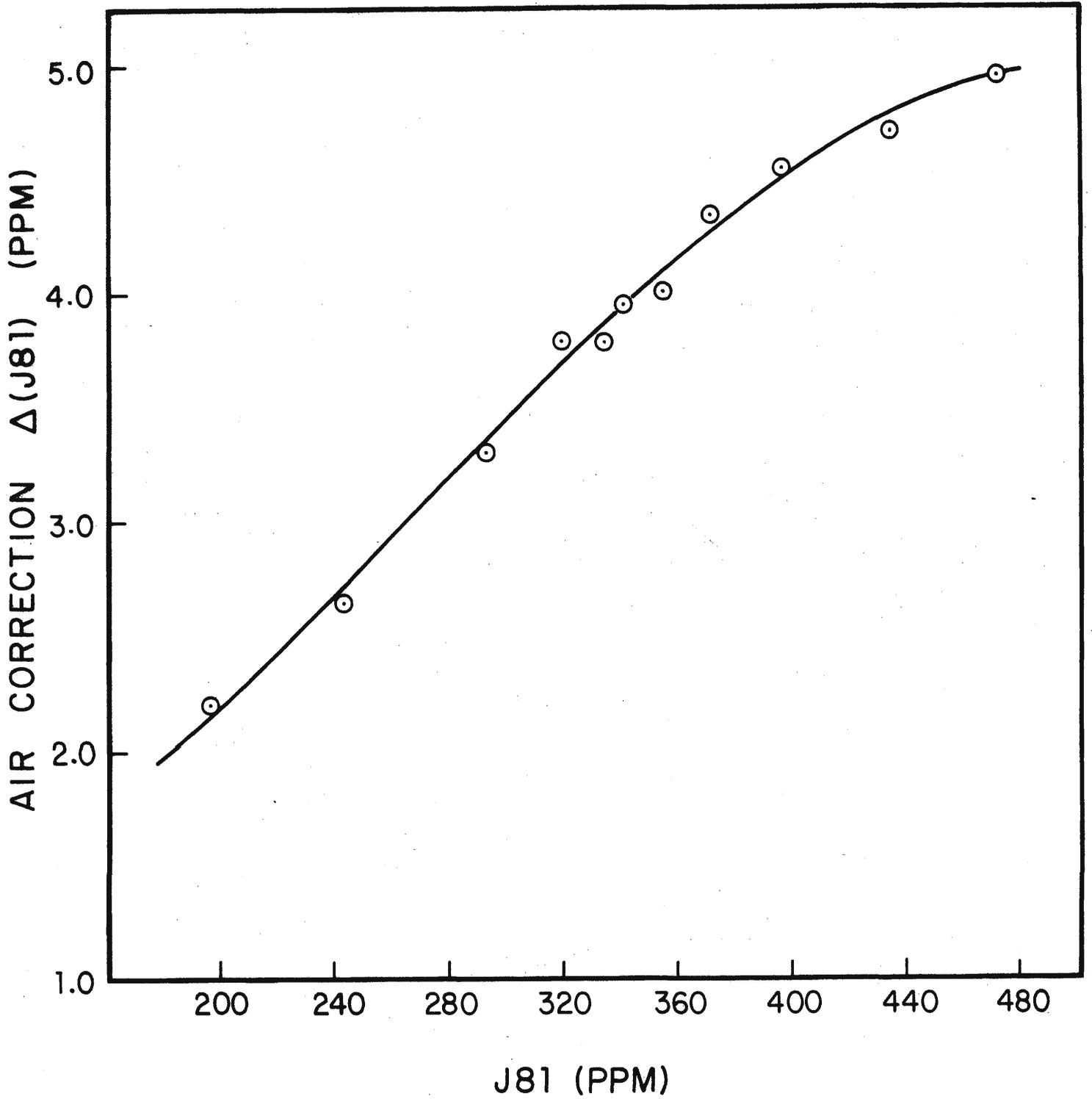
Fig. 2. Air correction obtained from 1980 and 1981 calibrations. Points are from CO<sub>2</sub>-in-air manometrically analyzed cylinders, compared to Scripps span gases on same day (see Table 6a).
