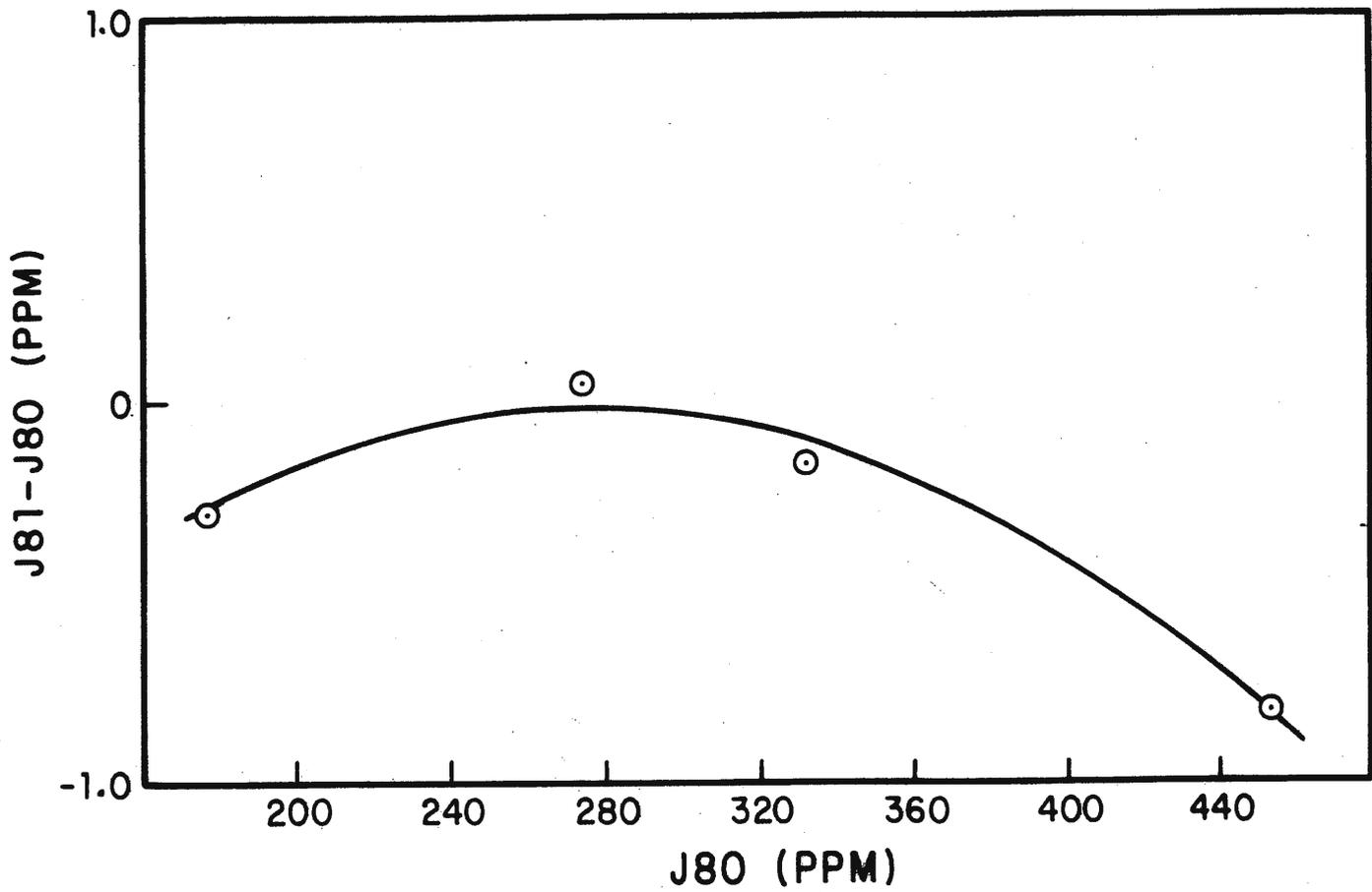
Fig. 1. System drift between 1980 and 1981 calibration periods (see Table 4). The equation for the curve is a quadratic least squares fit and is given in the text as equation (2).
