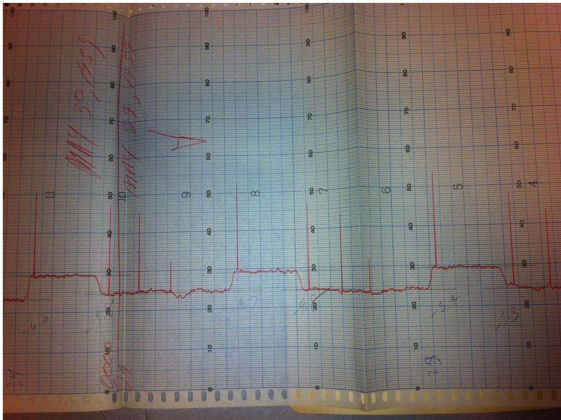
**Figure 3.** Example of a chart trace showing APC voltages. Spikes are inlet-switching events. Pencil marks are from 'lineout' readings with voltage differences listed. Time proceeds right to left.
