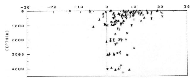
**Figure 4.** The difference (in  $\mu$ mol/kg) between titrimetric measurements of TCO<sub>2</sub> in seawater, and the gas extraction/ manometric data of Keeling, as achieved during the TTO program in 1981 [*Brewer et al.*, 1985]. The agreement is about one order of magnitude improved over that obtained during the 1969 Geosecs test cruise (Figure 2). The increased difference in the upper ocean values has not yet been satisfactorily explained. From *Brewer et al.* [1986].
