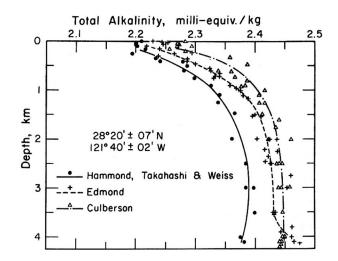
Figure 3. The alkalinity profile measured at the 1969 Geosecs test station [Takahashi et al., 1970]. The determination of alkalinity necessarily involves a titration procedure. The spread of values obtained was approximately 50 µeq/kg, much as was observed for the TCO<sub>2</sub> determination. Taken together, these two results gave serious concern as to whether the aims of the program could be achieved.
