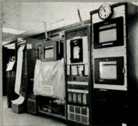
CO 2 instruments (left) in the new observatory building 1978, with meteorological and solar radiation strip charts (right).
